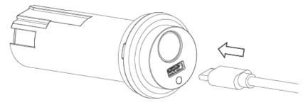
\*The battery pack will only begin charging if it is removed from the device and charged on a standalone basis.
